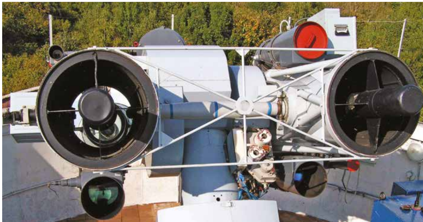
The Sazhen quantum optical system, based on laser meter, measures distances and angular outputs of the satellites
